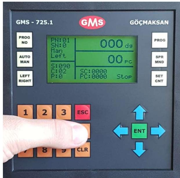
9. In order to use machine right and right bending angles, please push 0 and then push foot pedal. (If you push pedal before pushing 0, machine can remain the bending at last where it bended. )
