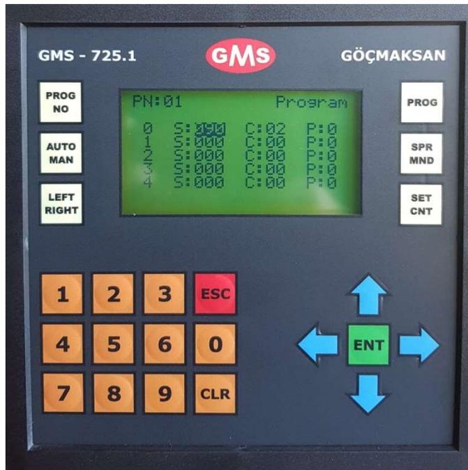
7. After entering angle on that part, please move to the bending number part with using right arrow . (C = Number of bendings) Do not enter anything on P part on screen. (You can move to different tabs with arrows )
