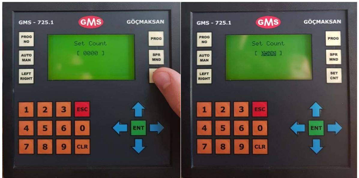
12. If you want to count the bended rebars on the machine you can use SET CNT button, After pushing SET CNT button please enter quantities.
