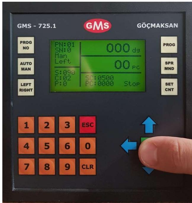
13. Please push ENT button & save it after entering rebar numbers to be bended. Machine will stop when its reach total bended rebar number.
