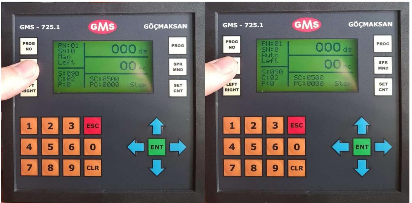
15. You can choose whether you are going to work on AUTO or MAN mode by choosing AUTO – MAN mode. You have to constalty press pedal until bending will be completed in manual mode, you have to only push once in auto mode.
