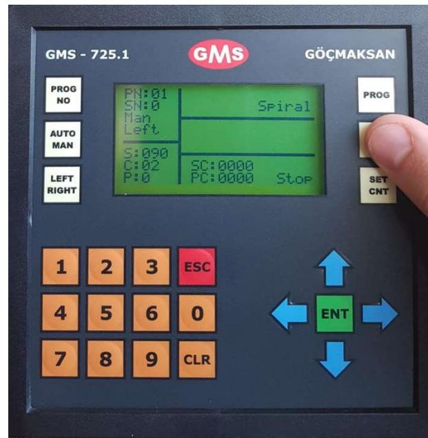
10. If you push SPR MND button, bending disc can constantly rotates, this function can be used on spiral bendings. (Please note that in order use this function you also have to use piral apparatus for this machine as well )
