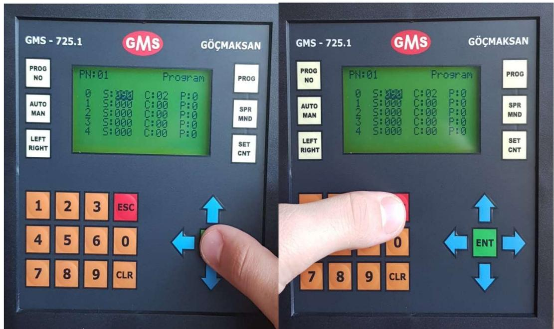
8. After entering all bending angles and diameters first push ENT and then ESC – with this you can save the program and move to the working page.
